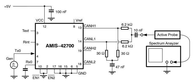
Figure 9. Basic Test Set-up for Electromagnetic Measurement
