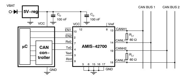
Figure 3. Application Diagram Dual-CAN
