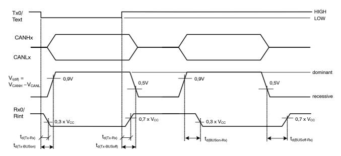
Figure 8. Timing Diagram for AC Characteristics
