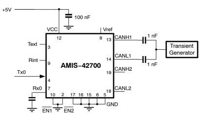
Figure 5. Test Circuit for Automotive Transients
