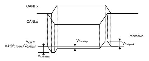
Figure 10. Common-mode Voltage Peaks (see measurement set-up Figure 9)
