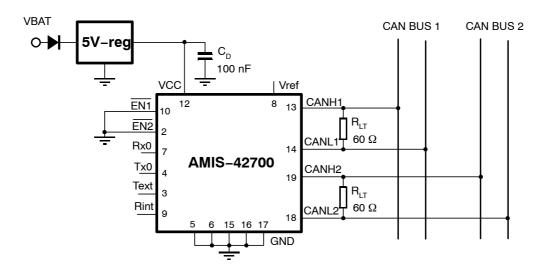
Figure 2. Application Diagram CAN-bus Repeater
