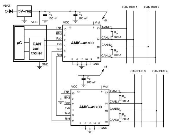
Figure 4. Application Diagram CAN-bus Extender
