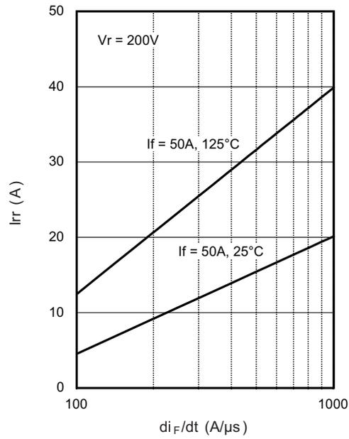
Fig. 9 - Typical Stored Current vs.  $di_F/dt$
