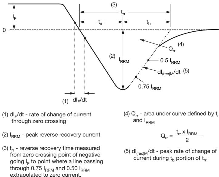
Fig. 11 - Reverse Recovery Waveform and Definitions
