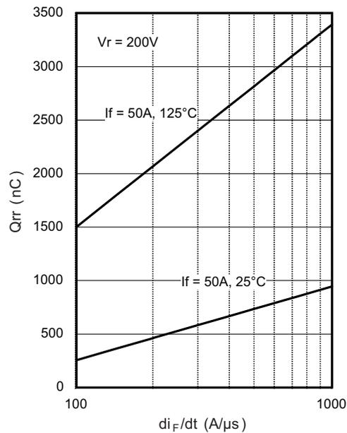
Fig. 7 - Typical Stored Charge vs.  $di_F/dt$
