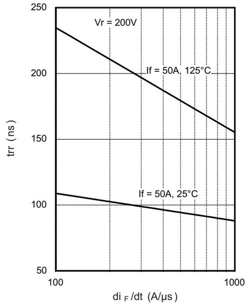
Fig. 6 - Typical Reverse Recovery Time vs.  $di_F/dt$
