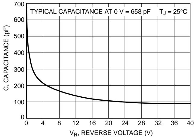
Figure 7. Typical Capacitance
