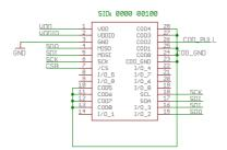
BMP280 shuttle board electrical layout
