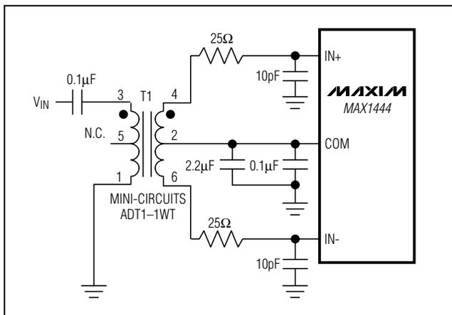
Figure 8. Using a Transformer for AC Coupling
