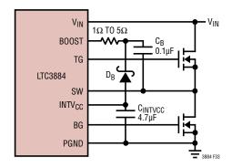
Figure 33. Boost Circuit to Minimize PWM Jitter
