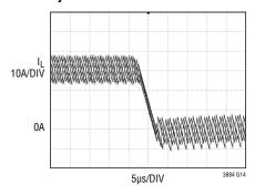
**Current Limit During an Output Short Condition**
