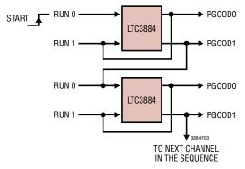
Figure 3. Event (Voltage) Based Sequencing
