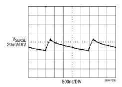
Figure 29b. Voltage Measured After the  $R_{SENSE}$  Filter
