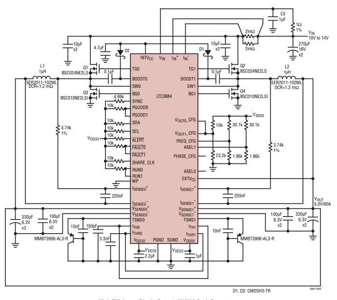
High Efficiency, Single-Output, 5V/60A Buck Converter
