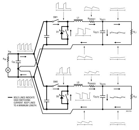
Figure 40b. Branch Current Waveforms
