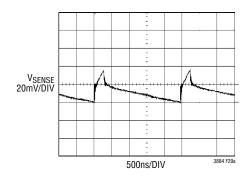
Figure 29a. Voltage Measured Directly Across R<sub>SENSE</sub>
