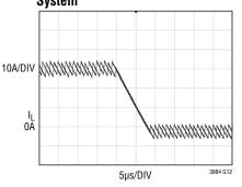
**Dynamic Current Sharing During** a Load Transient in a 4-Phase System
