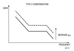
Figure 37. Error Amp gm Adjust
