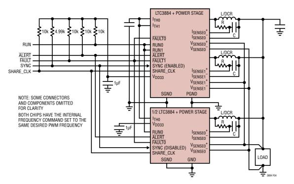
Figure 4. Load Sharing Connections for 3-Phase Operation
