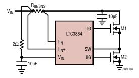
Figure 36. Low Noise Input Current Sense Circuit
