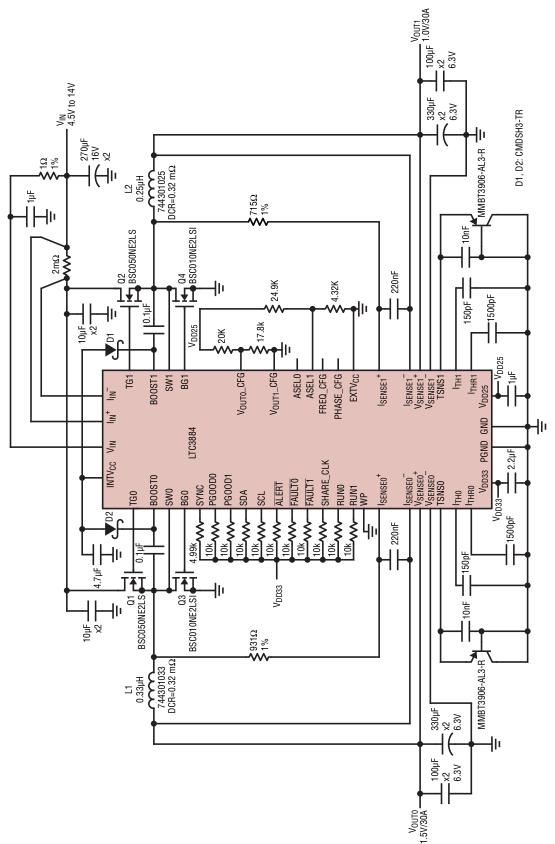
High Efficiency, Dual-Output 1.5V/30A and 1.0V/30A, Buck Converter
