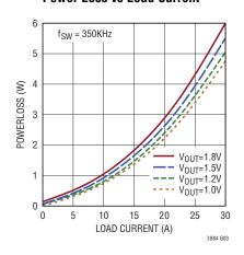
**Power Loss vs Output Current**
