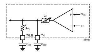
Figure 36. Programmable Loop Compensation
