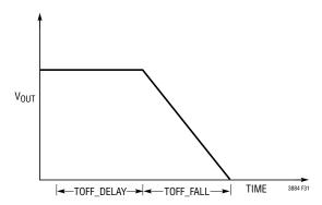
Figure 31. TOFF\_DELAY and TOFF\_FALL
