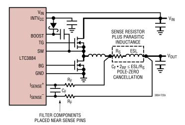
Figure 28b. Resistor Current Sense Circuit
