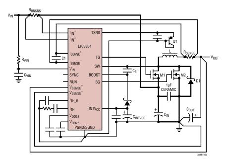
Figure 40a. Recommended Printed Circuit Layout Diagram, Single Phase Shown
