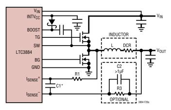
Figure 28a. Inductor DCR Current Sense Circuit
