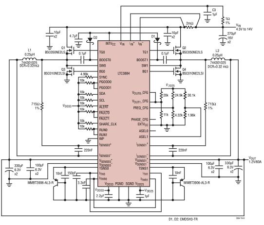
High Efficiency, Single-Output, 1.2V/60A Buck Converter
