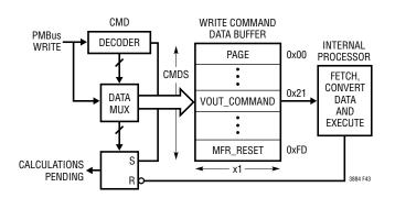
Figure 43. Write Command Data Processing
