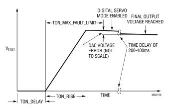
Figure 30. Timing Controlled Vout Rise
