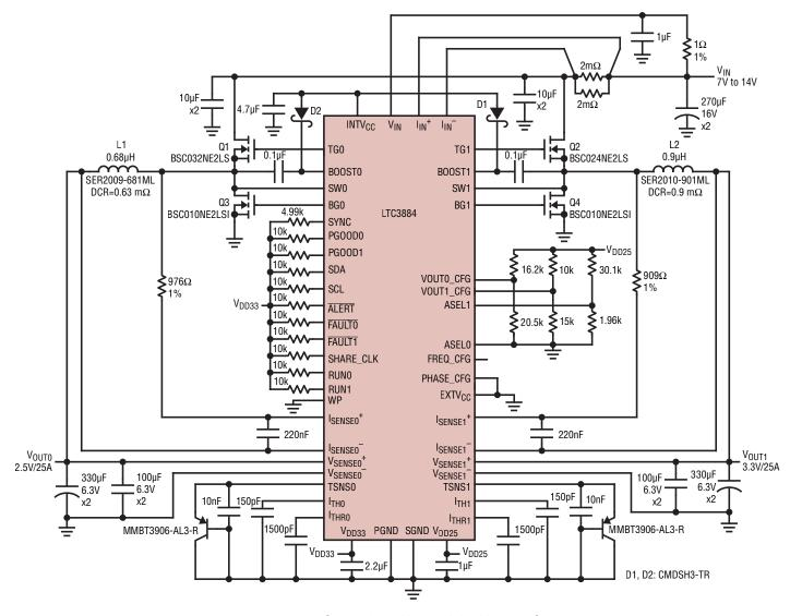
High Efficiency, Dual-Output, 2.5V/30A and 3.3V/30A Buck Converter
