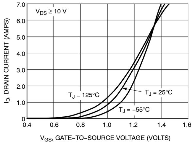
**Figure 2. Transfer Characteristics**
