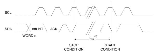
Note: 1. The write cycle time t<sub>WR</sub> is the time from a valid stop condition of a write sequence to the end of the internal clear/write cycle.
