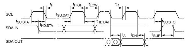
Figure 23. Physical Device Address (A<sub>0</sub>) Pin Timing
