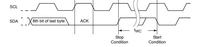
Figure 25. Write Protect (WP) Pin Timing During Slave Address
