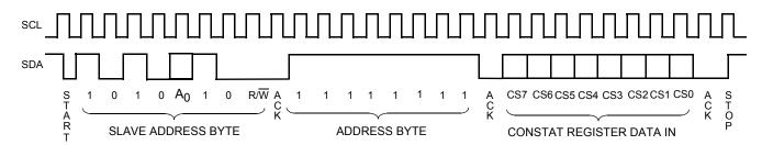
Figure 18. CONSTAT Register Write Command Sequence
