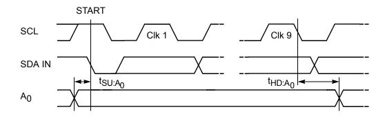
Figure 24. Write Cycle Timing
