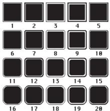
commands draw box frame and draw touchkeys. There are also three special borders in various colors for using with bargraph commands (no:101..107, 111..117 and 121..127). All of them can be used in various sizes via coordinates. The frames 1..20 are split into 3 segments: the outer frame, inner frame and filling. Each segment will get an individual colour for normal and for selected state. This will give the user
