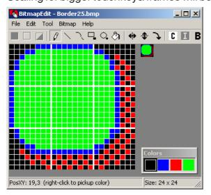
segments. This makes it necessary to keep the 8x8 size in every case. If 4-color bitmaps are used (as the preloaded border 1..20) the color can be set individually (the first color is always transparent and is not used by the eDIP). It is also possible to define full colored border (as the preloaded border for bargraphs 101...127).With the
