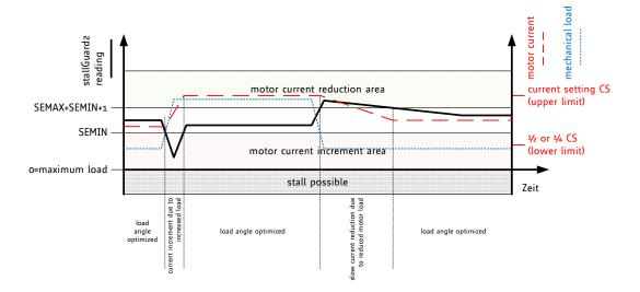
Figure 7.2 Motor current control via coolStep adapts motor current to motor load
