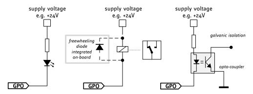
Figure 4.5 Possible circuits for GPO
