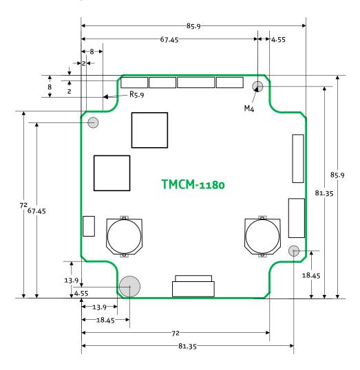
Figure 4.1 Dimensions of TMCM-1180 and mounting holes
