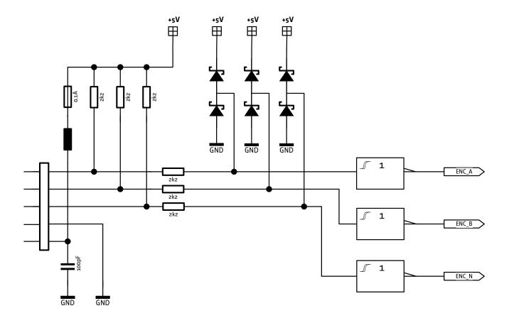
Figure 4.13 Internal circuit of encoder interface
