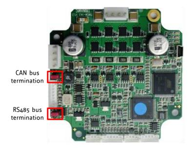
Figure 5.1 RS485 and CAN bus termination
