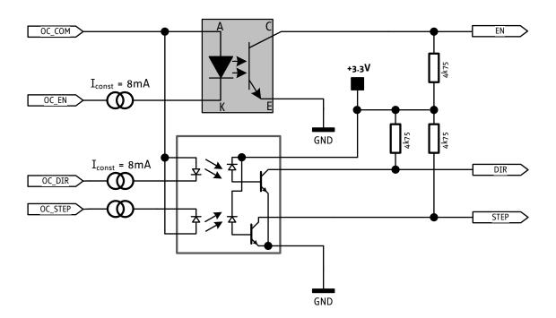
Figure 4.12 Internal circuit of the Step/Dir interface
