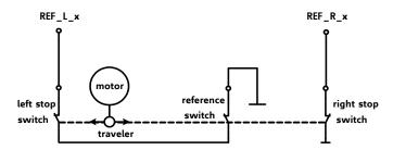
Figure 4.10 Limit switch and reference switch
