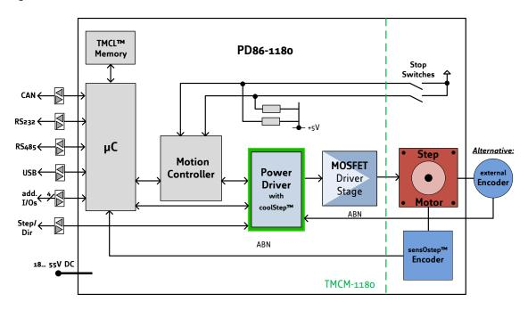
Figure 7.1 Main parts of the PD86-1180
