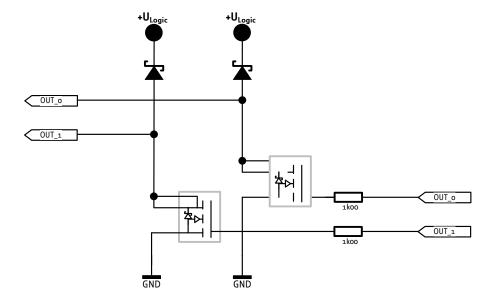
Figure 4.6 Internal circuit of the outputs
