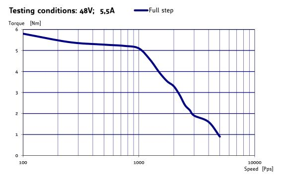
Figure 4.3 QSH8618-96-55-700 speed vs. torque characteristics
