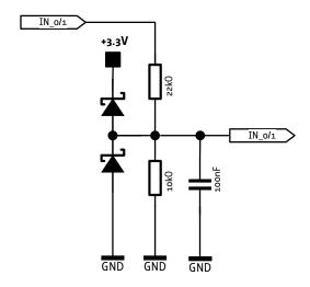
Figure 4.8 Internal circuit of the inputs
