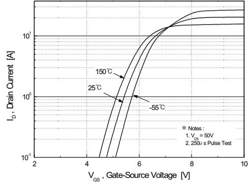
Figure 2. Transfer Characteristics
