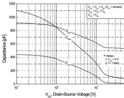
Figure 5. Capacitance Characteristics
