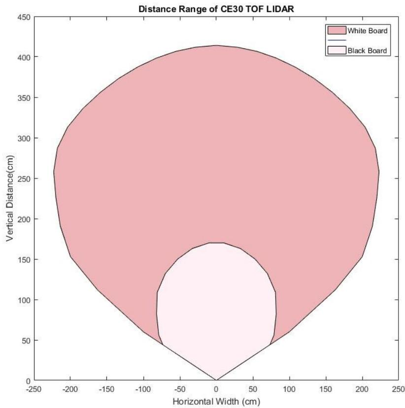
Figure 7 Optimized Detecting Area for Obstacle Avoidance Application
