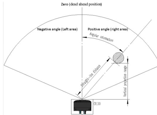
Figure 8 Testing Data Illustration (Top View)
