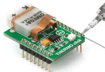
Turn the board upward again. Make sure to align the headers so that they are perpendicular to the board, then solder the pins carefully.
