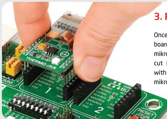
Once you have soldered the headers your board is ready to be placed into desired mikroBUS™ socket. Make sure to align the cut in the lower-right part of the board with the markings on the silkscreen at the mikroBUS™ socket. If all of the pins are aligned correctly, push the board all the way into the socket.
