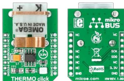
THERMO Click™ is an accessory board in **mikroBUS™** form factor. It's a compact solution for adding thermocouple to your device. It features **MAX3185K** thermocouple-to-digital converter as well as **PCC-SMP** connector for K-type thermocouple probes. THERMO Click™ communicates with the target board via SPI interface (Read-only). The board is designed to use 3.3V power supply only. It has a LED diode (GREEN) that indicates the presence of power supply.
