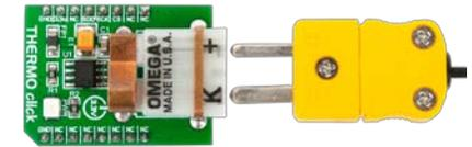
In order to use THERMO Click™ board you need to connect the appropriate K-type thermocouple probe (not included in the package) into the PCC-SMP connector, as shown in figure above.
