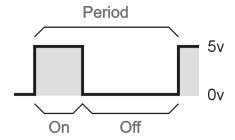
The PWMPAL gives the program control of the on- and off-time values, hence giving control of the output frequency and duty cycle. In the PWMPAL, the on and off times are specified with 16-bit values in units of 25 microseconds (0.000025 seconds). Using the formula:
