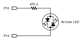
Notice that due to the differences between relative [perceived] brightness of the green and red LEDs, the AC waveform is set such that the duty cycle favors the green LED.
