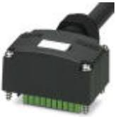
Connector hood, For use in Sensor/actuator box, Connection method: M12-SPEEDCON-socket Plastic, Number of slots: 4, Slot assignment: Single, Status indication: No; Master cable connection: Pluggable screw connection 180°, Cable length: 10 m, Shielding: No
