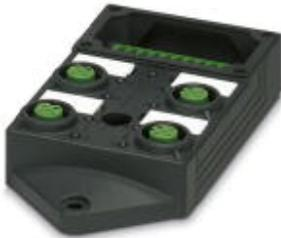
Sensor/actuator box header, Connection method: M12-SPEEDCON-socket Plastic, Number of slots: 4, Number of positions: 4, Slot assignment: Single, Status indication: Yes, pnp; Master cable connection: Pluggable screw connection, Shielding: No
