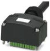
Connector hood, For use in Sensor/actuator box, Connection method: M12-SPEEDCON-socket Plastic, Number of slots: 4, Slot assignment: Single, Status indication: No; Master cable connection: Pluggable screw connection 180°, PUR/PVC, Cable length: 0.5 m ... 50 m, Shielding: No
