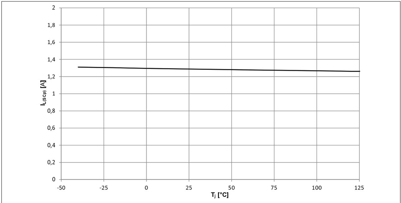
**Figure 30** Typical Initial Peak Short Circuit Current Limit vs  $T_j$
