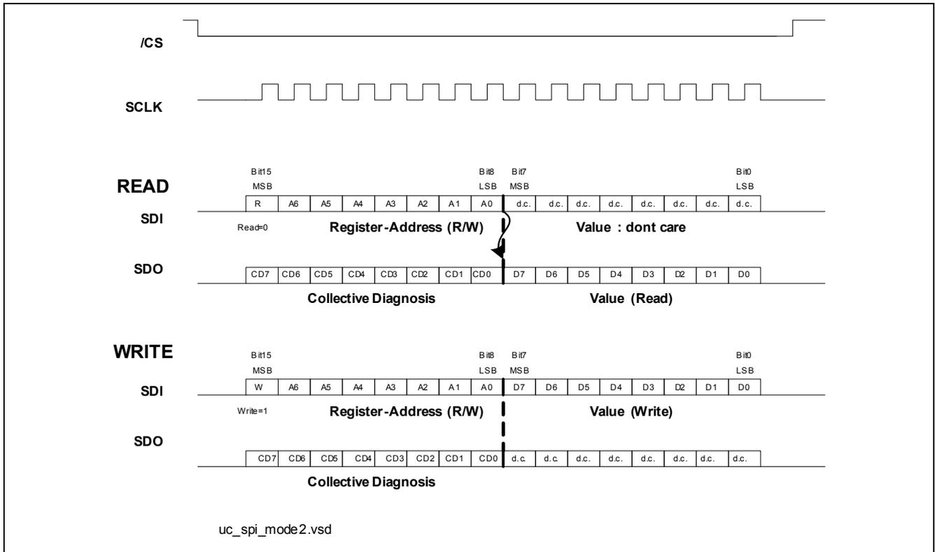
Figure 14 SPI Mode 2, MS0 = 0, MS1 = 1
