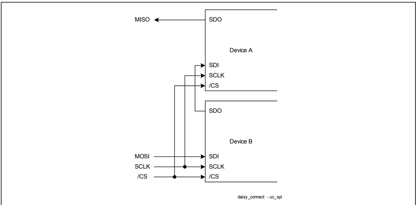
**Figure 16 Connecting Two Devices for Daisy Chain Mode**
