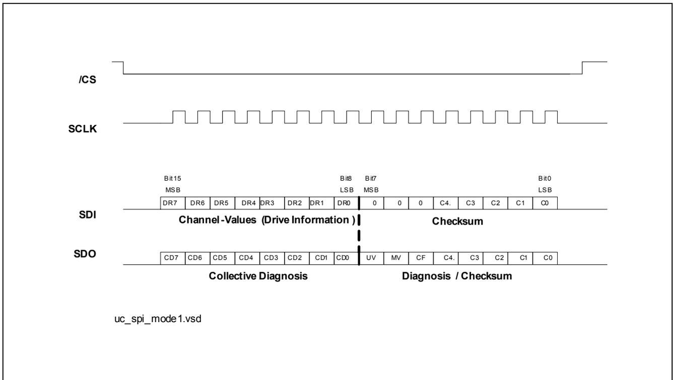
Figure 13 SPI Mode 1, MS0 = 1, MS1 = 0, Daisy Chain Supported
