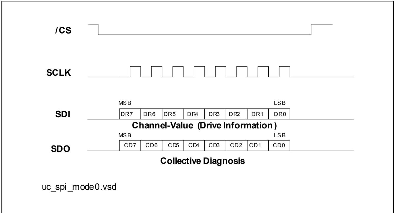
Figure 12 SPI Mode 0, MS0 = 0, MS1 = 0, Daisy Chain Supported
