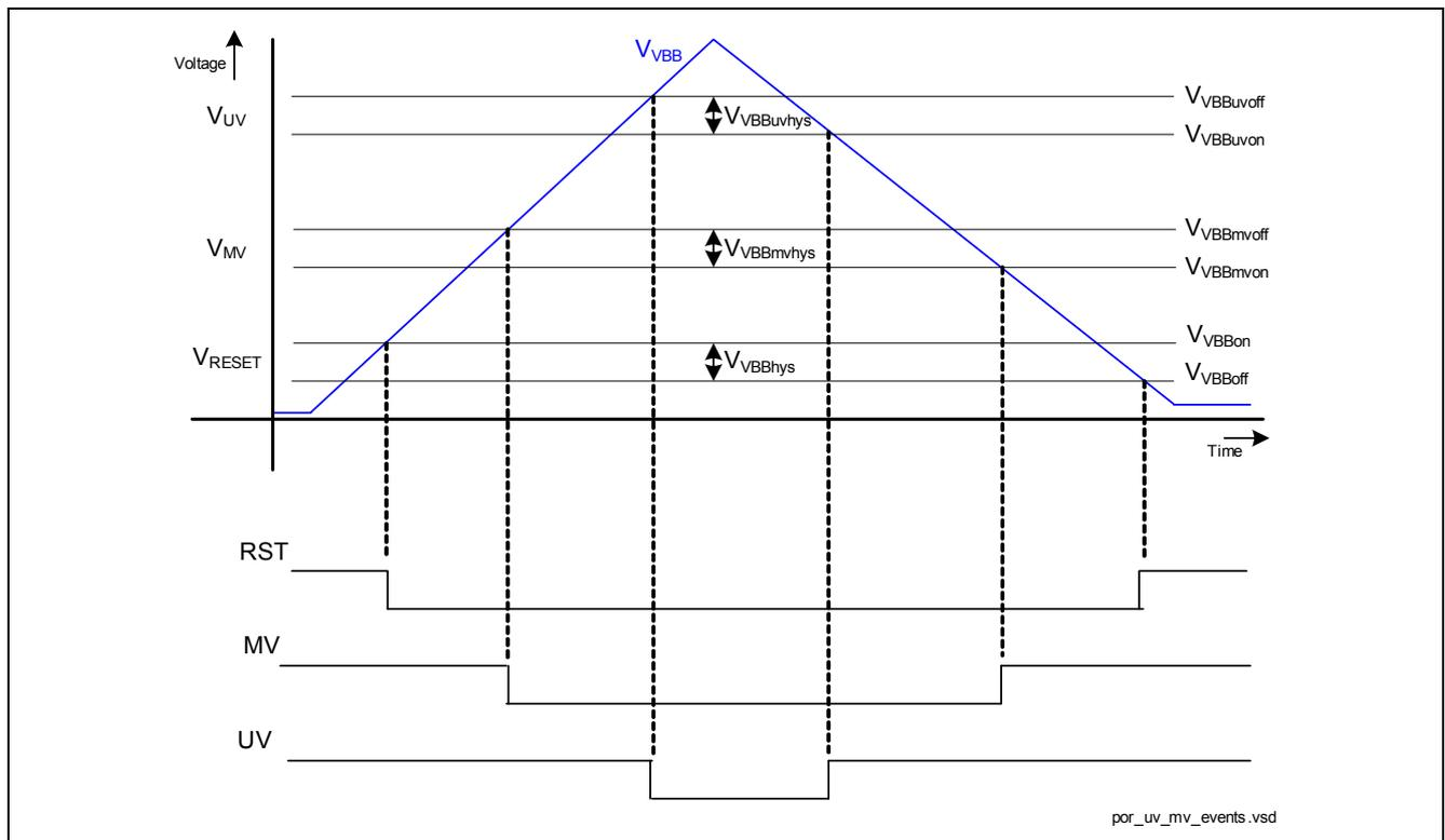
**Figure 22 Start Up Procedure of the Power Chip**
