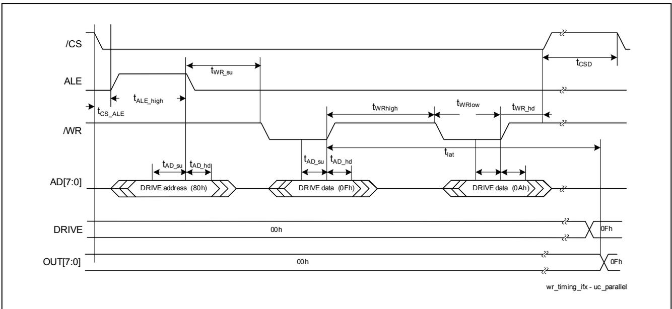
**Figure 8** Timing by Parallel Write Access (e.g. **DRIVE** Register)
