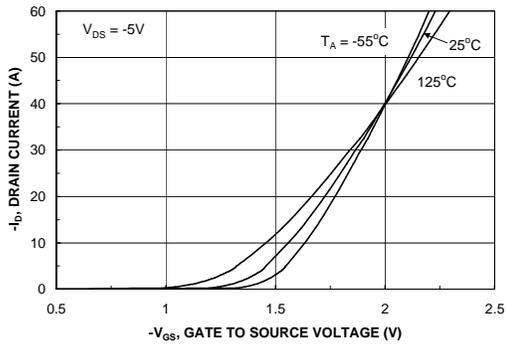
Figure 5. Transfer Characteristics.
