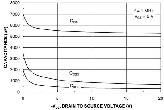
Figure 8. Capacitance Characteristics.
