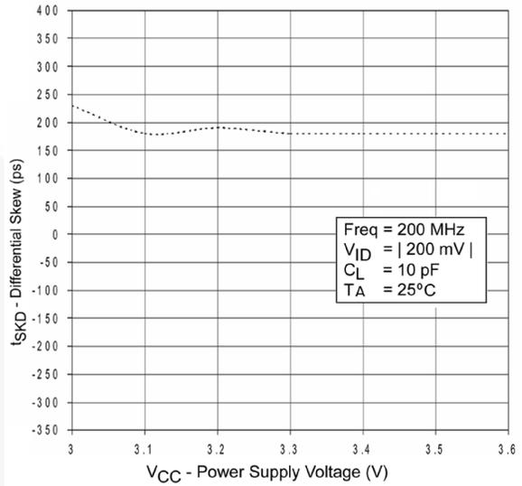
Figure 12. Differential Skew vs. Power Supply Voltage
