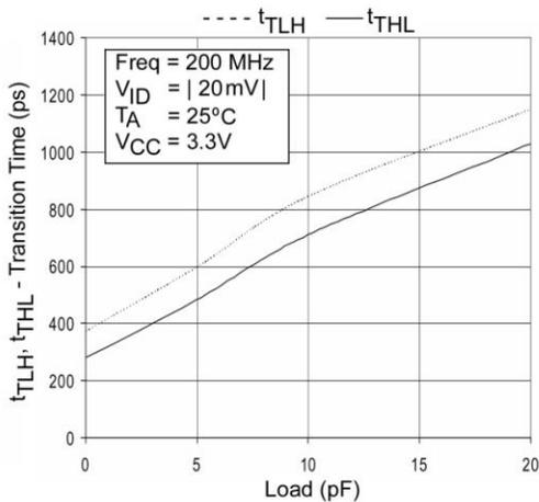
**Figure 21. Transition Time vs. Load**
