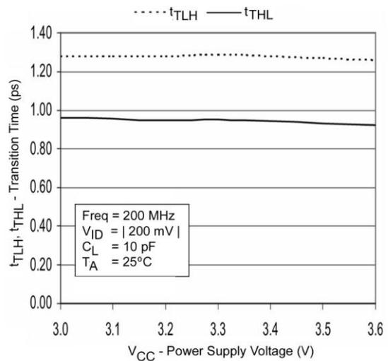
Figure 16. Transition Time vs. Power Supply Voltage
