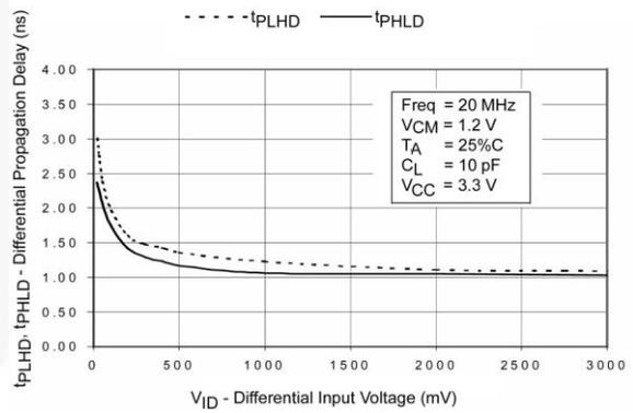
Figure 14. Differential Propagation Delay vs. Differential Input Voltage
