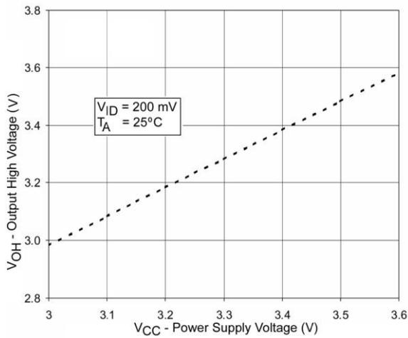
**Figure 5. Output High Voltage vs. Power Supply Voltage**
