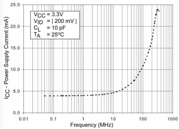
**Figure 8. Power Supply Current vs. Frequency**
