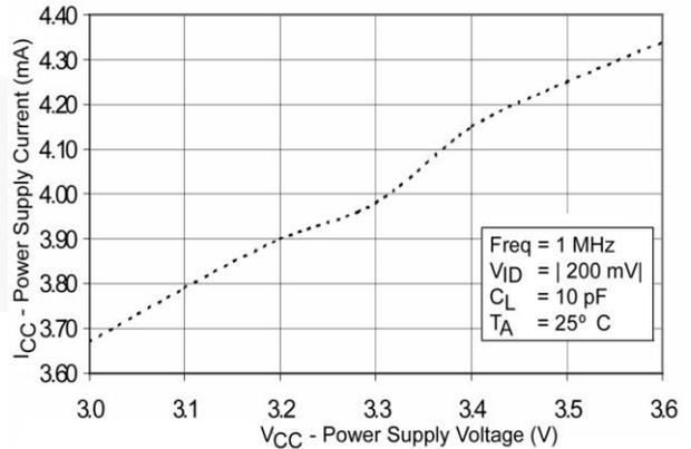
**Figure 22. Power Supply Current vs. Power Supply Voltage**
