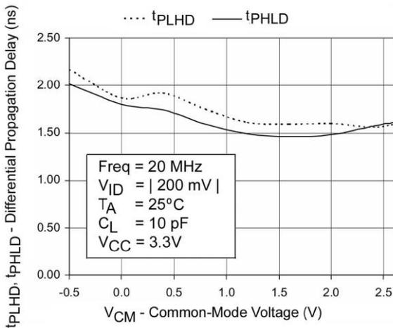
Figure 15. Differential Propagation Delay vs. Common-Mode Voltage
