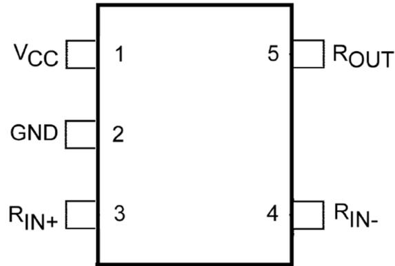
Figure 2. Pin Configuration
