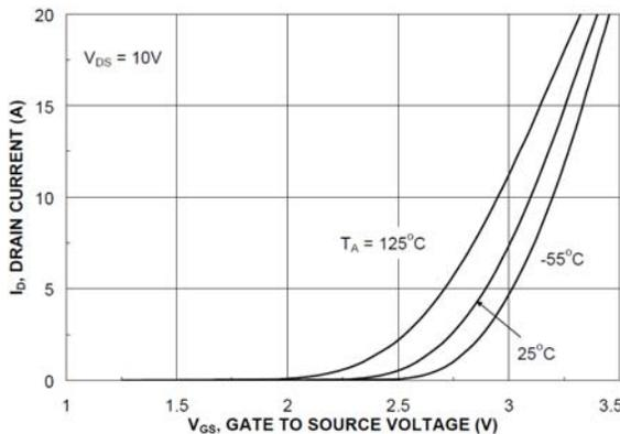
Figure 5. Transfer Characteristics
