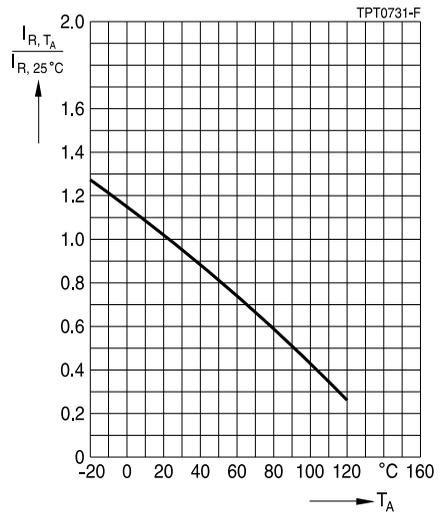
**Characteristics (typical) for  $T_{ref} = 130\text{ }^{\circ}\text{C}$**
