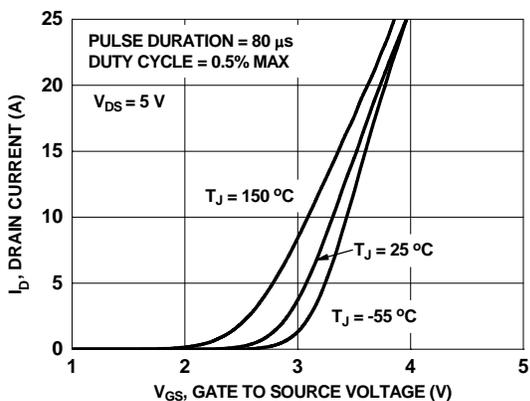
Figure 5. Transfer Characteristics
