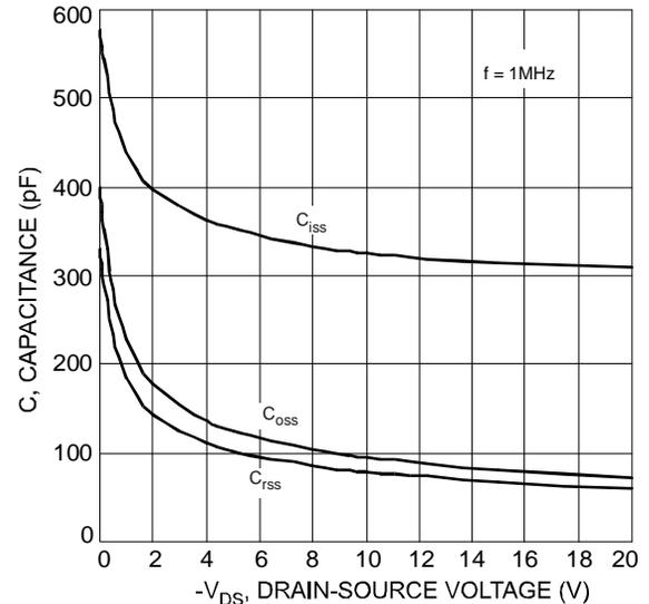
Fig. 6: Typical Capacitance
