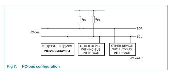
The P89V660/662/664 CPU interfaces with the I<sup>2</sup>C-bus through four Special Function Registers (SFRs): S1CON (primary I<sup>2</sup>C-bus Control Register), S1DAT (primary I<sup>2</sup>C-bus Data Register), S1STA (primary I<sup>2</sup>C-bus Status Register), and the S1ADR (primary I<sup>2</sup>C-bus Slave Address Register).
