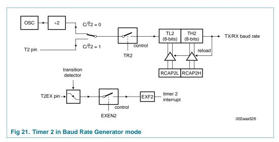
The baud rate generation mode is like the auto-reload mode, when a rollover in TH2 causes the Timer 2 registers to be reloaded with the 16-bit value in registers RCAP2H and RCAP2L, which are preset by software.
