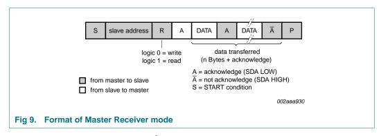
After a repeated START condition, I<sup>2</sup>C-bus may switch to the Master Transmitter mode.
