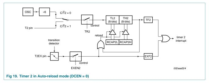
In this mode, there are two options selected by bit EXEN2 in T2CON register. If EXEN2 = 0, then Timer 2 counts up to 0FFFFH and sets the TF2 (Overflow Flag) bit upon overflow. This causes the Timer 2 registers to be reloaded with the 16-bit value in RCAP2L and RCAP2H. The values in RCAP2L and RCAP2H are preset by software means.
