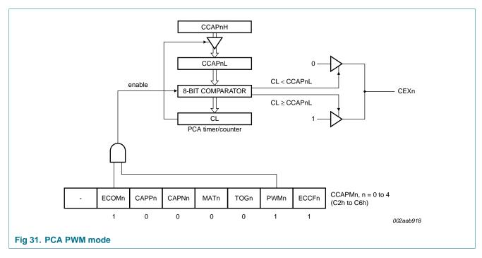
All of the modules will have the same frequency of output because they all share one and only PCA timer. The duty cycle of each module is independently variable using the module's capture register CCAPnL. When the value of the PCA CL SFR is less than the
