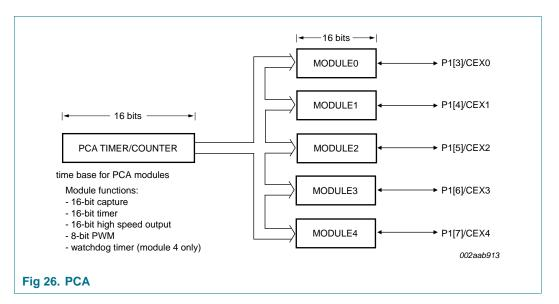
In the CMOD SFR there are three additional bits associated with the PCA. They are CIDL which allows the PCA to stop during Idle mode, WDTE which enables or disables the Watchdog function on module 4, and ECF which when set causes an interrupt and the PCA overflow flag CF (in the CCON SFR) to be set when the PCA timer overflows.
