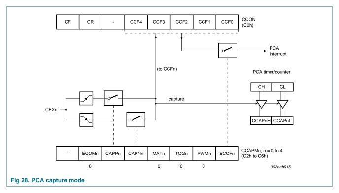
If the CCFn bit for the module in the CCON SFR and the ECCFn bit in the CCAPMn SFR are set then an interrupt will be generated.
