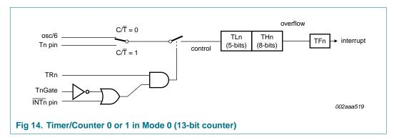
In this mode, the Timer register is configured as a 13-bit register. As the count rolls over from all 1s to all 0s, it sets the Timer interrupt flag TFn. The count input is enabled to the Timer when TRn = 1 and either GATE = 0 or INTn = 1. (Setting GATE = 1 allows the Timer to be controlled by external input INTn, to facilitate pulse width measurements). TRn is a control bit in the Special Function Register TCON (Figure 5). The GATE bit is in the TMOD register.
