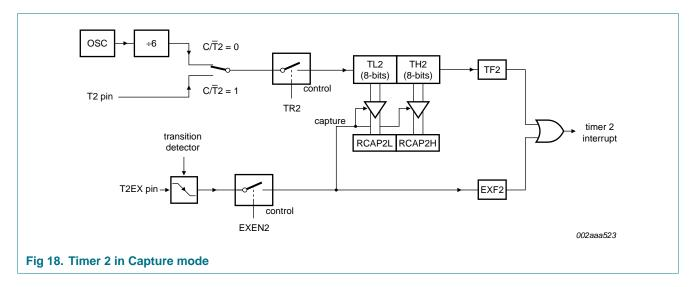
This bit can be used to generate an interrupt (by enabling the Timer 2 interrupt bit in the IEN0 register). If EXEN2 = 1, Timer 2 operates as described above, but with the added feature that a 1- to -0 transition at external input T2EX causes the current value in the Timer 2 registers, TL2 and TH2, to be captured into registers RCAP2L and RCAP2H, respectively.
