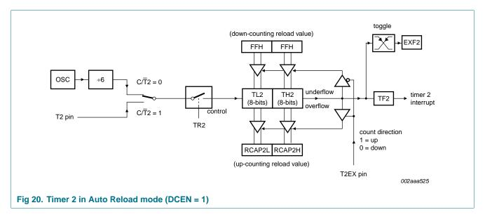
When a logic 0 is applied at pin T2EX this causes Timer 2 to count down. The timer will underflow when TL2 and TH2 become equal to the value stored in RCAP2L and RCAP2H. Timer 2 underflow sets the TF2 flag and causes 0FFFFH to be reloaded into the timer registers TL2 and TH2. The external flag EXF2 toggles when Timer 2 underflows or overflows. This EXF2 bit can be used as a 17th bit of resolution if needed.
