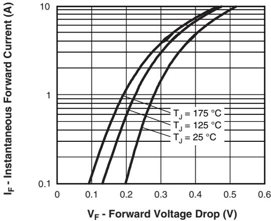
Fig. 1 - Typical Forward Voltage Drop Characteristics (Per Leg)
