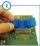
Place HS over the installed FC so that the "horseshoe" tabs of the FC fit within the HS' notches.
