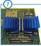
Shown above the is the HS, FC and SC assembly properly seated over the component.
