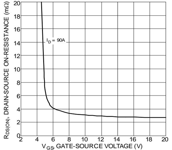
Figure 4 Typical Drain-Source On-Resistance vs. Gate-Source Voltage
