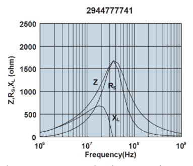
Impedance, reactance, and resistance vs. frequency.
