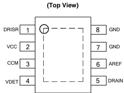
Note: The DRAIN pin of internal MOSFET is exposed PAD, which is at the bottom of IC (the dashed box). The secondary current should flow from GND(pin 7,8) to the exposed PAD.
