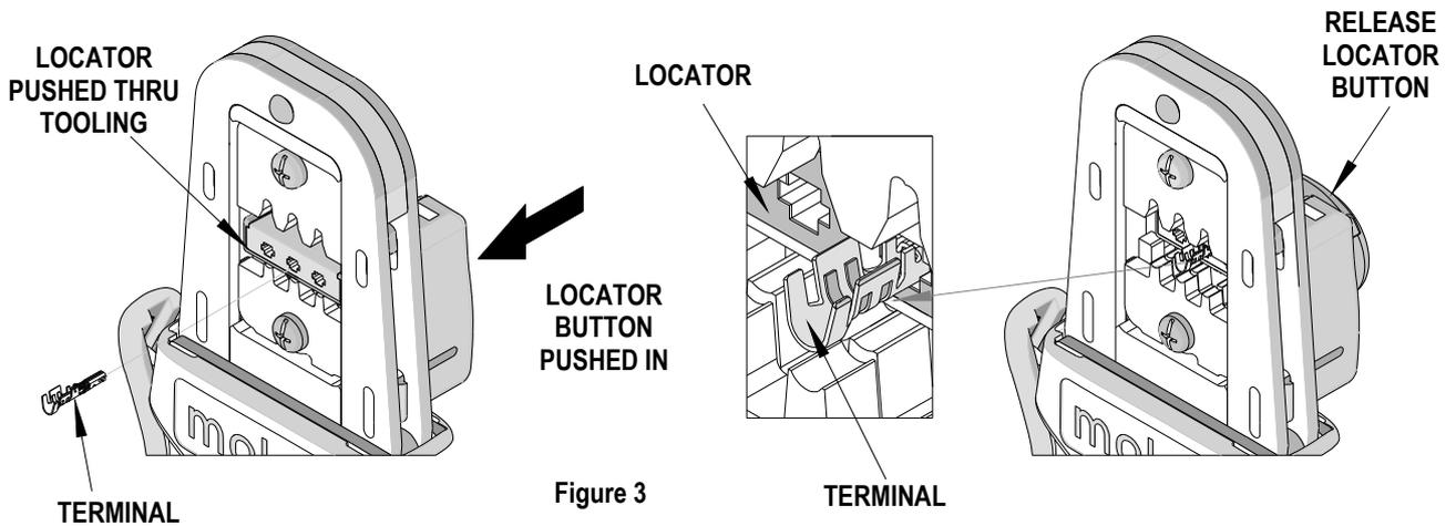
4. Release the locator button, allowing the locator to return to the crimping position.
