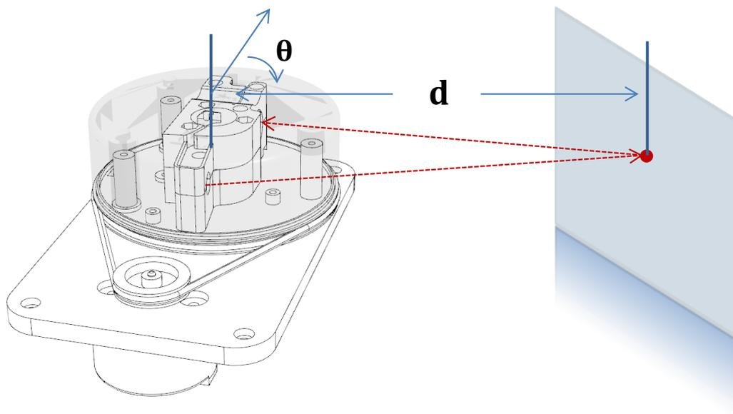
The high-speed ranging scanner system is mounted on a spinning rotator with a build-in angular encoding system. During rotating, a 360 degree scan of the current environment will be performed.
