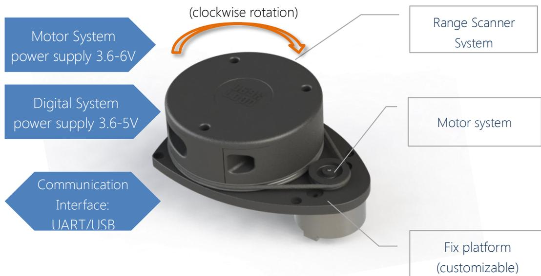
RPLIDAR comes with a speed detection and adaptive system. The system will adjust frequency of laser scanner automatically according to motor speed. And host system can get RPLIDAR's real speed through communication interface.
