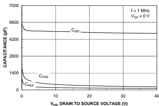
Figure 8. Capacitance Characteristics.
