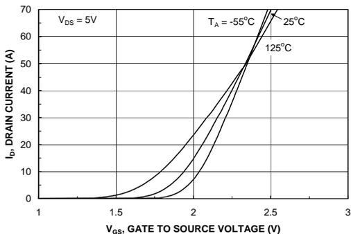
Figure 5. Transfer Characteristics.
