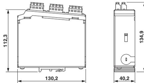
DIN rail splice box 6x LC quad OM2, fully mounted ready to splice
