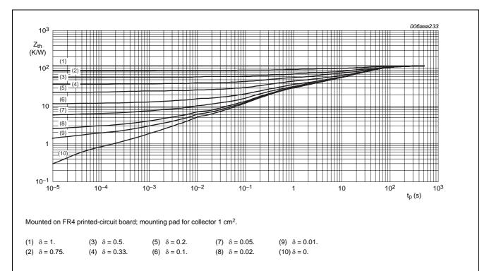
Fig.4 Transient thermal impedance as a function of pulse time; typical values.
