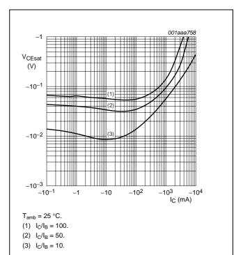
Fig.11 Collector-emitter saturation voltage as a
