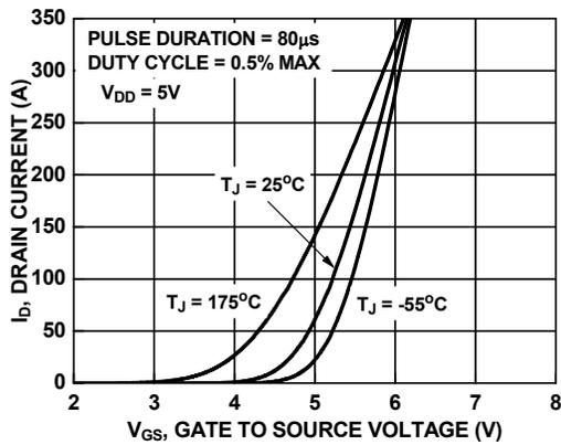
Figure 7. Transfer Characteristics
