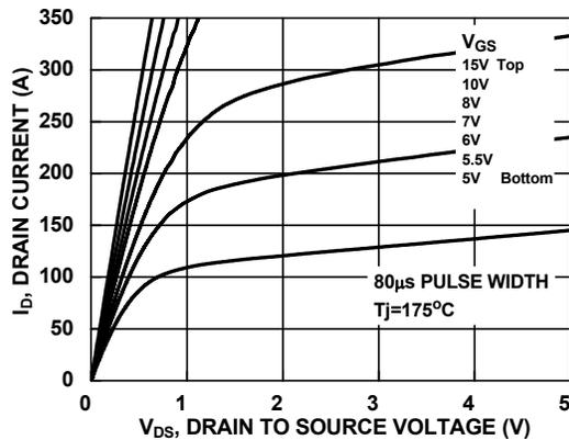
Figure 10. Saturation Characteristics
