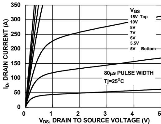
Figure 9. Saturation Characteristics
