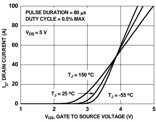
Figure 5. Transfer Characteristics
