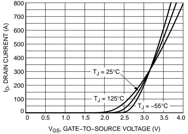
Figure 2. Transfer Characteristics
