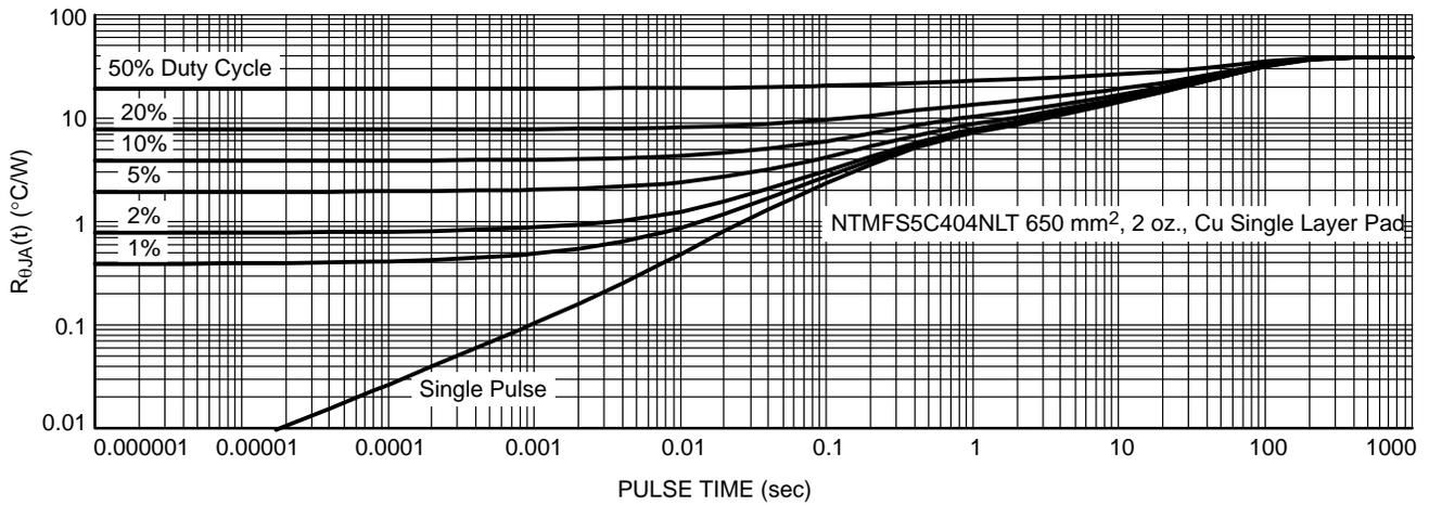
Figure 13. Thermal Characteristics
