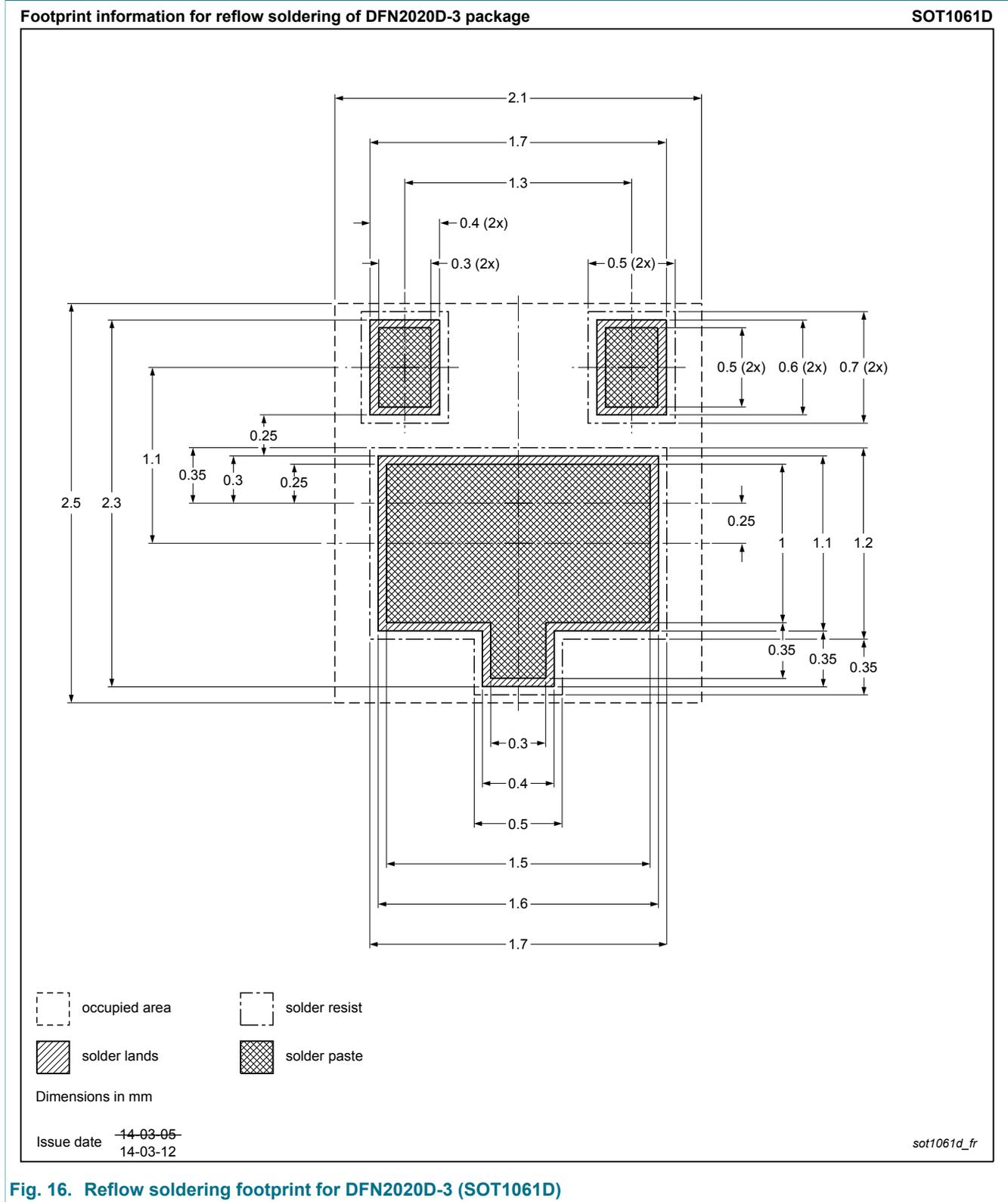
Fig. 16. Reflow soldering footprint for DFN2020D-3 (SOT1061D)
