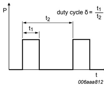
Fig. 14. Duty cycle definition
