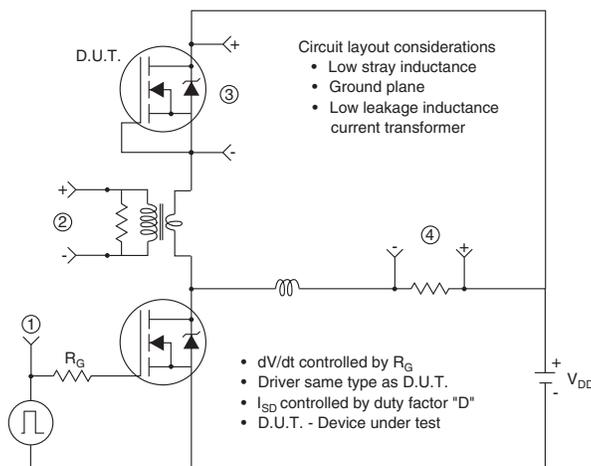
Fig. 13c - Peak Diode Recovery dV/dt Test Circuit
