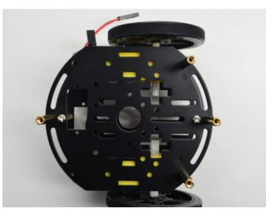
Screw in the chassis layer by attaching to the brass standoffs
