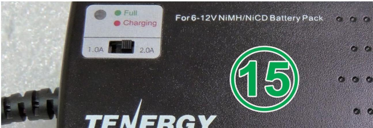
1. Switch the current of “⑮ Battery Charger” to 2.0A.
