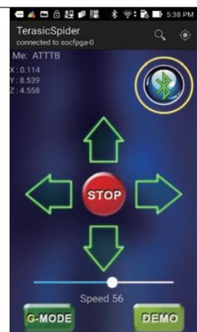
13. The four Arrow Buttons control the Spider movement in four directions (default mode). Spider's movement speed can be controlled by the Speed Slider. Slide left to slow down the Spider; Slide right to speed up.
