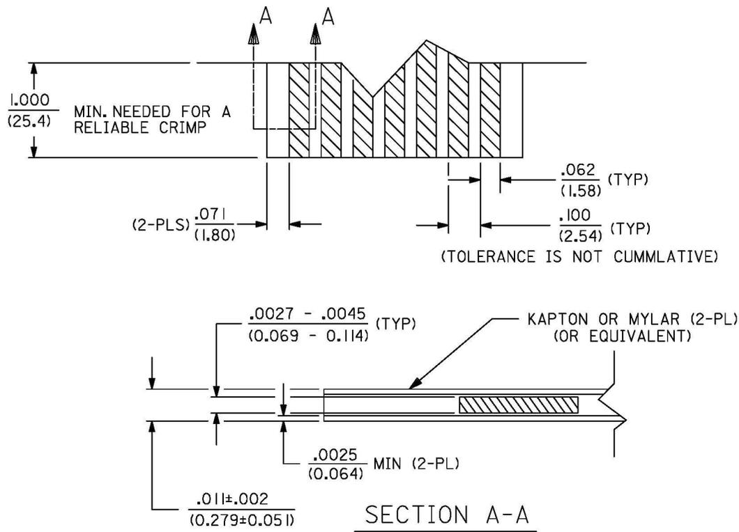
**2.2.4.1.1** Cable length required to successfully terminate assemblies in Molex equipment is 1.00/(25.4) minimum.
