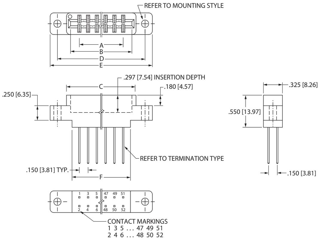
Tolerances on non-critical dimensions may vary slightly due to shrinkage differential per insulator material; Consult factory.
