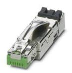
RJ45 connector, contact inserts: x , degree of protection: IP20, number of positions: 6, 100 Mbps, CAT5 (IEC 11801:2002), material: Zinc die-cast, connection method: IDC fast connection, connection cross section: AWG 26- 24, cable outlet: straight, High degree of resistance to vibration; 360° shielding; one-piece design; special tool-free assembly
