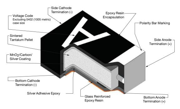
Fig. 1 - Leadframeless Molded Capacitors, All Types
