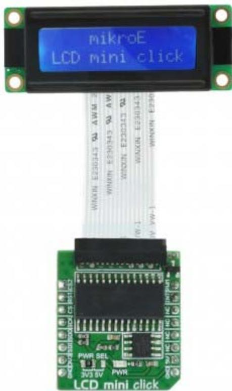
**LCD mini click** displays 2x16 monochrome characters on an LMB162XFW LCD display. It features the MCP23S17 port expander and the MCP4161 digital potentiometer, both from Microchip. LCD mini click is designed to run on either 3.3V or 5V power supply. It communicates with the target microcontroller over SPI interface and the following pins on the mikroBUS™ line: PWM, INT, RST, AN.
