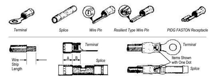
"A" is Insulation Barrel, "B" is Wire Barrel
