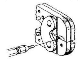
"GO" Gage Must Pass Completely Through the Die Closure
