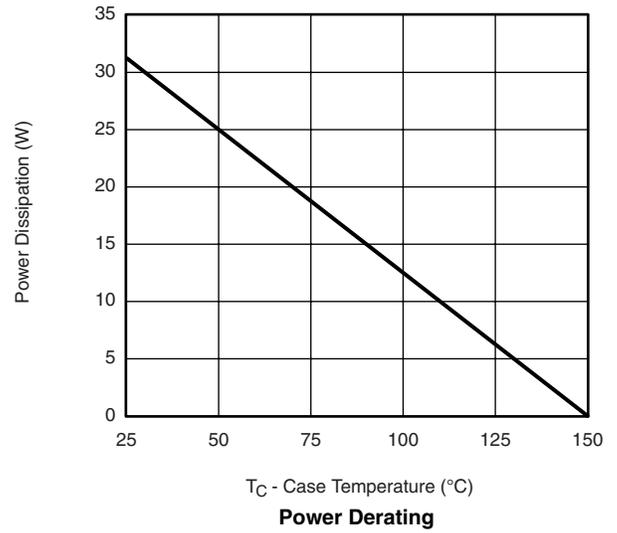
\* The power dissipation  $P_D$  is based on  $T_{J(max)} = 150\text{ °C}$ , using junction-to-case thermal resistance, and is more useful in settling the upper dissipation limit for cases where additional heatsinking is used. It is used to determine the current rating, when this rating falls below the package limit.
