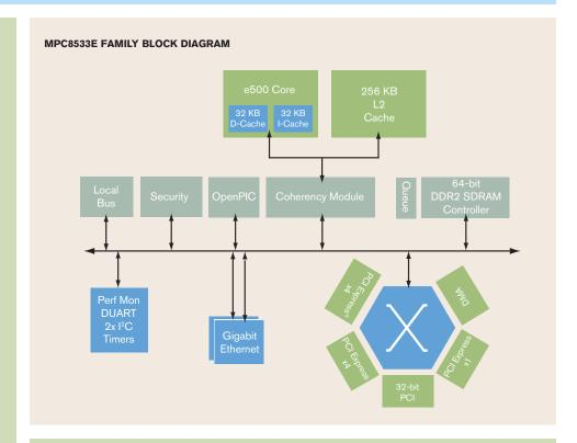
The MPC8533E processor offers a wide range of high-speed connectivity options, including Gigabit Ethernet (GigE) and multiple PCI Express® connections.
