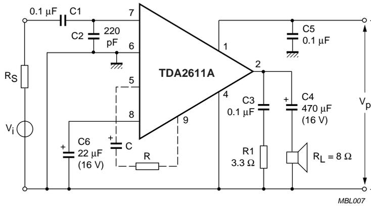
Fig.3 Test circuit; pin 3 not connected.
