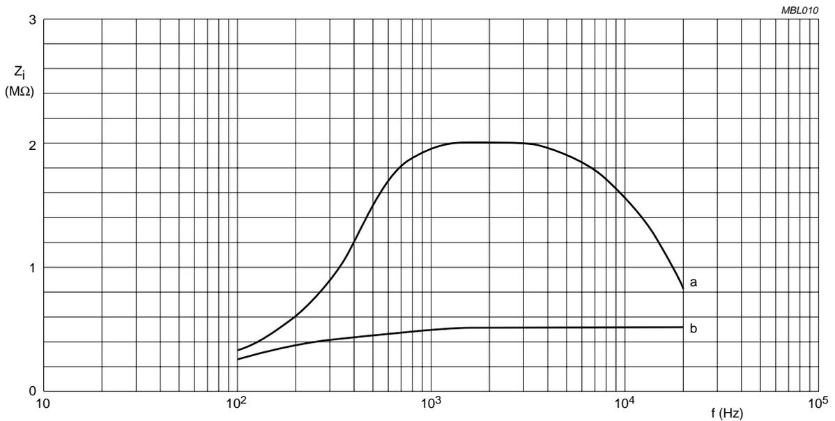
Fig.6 Input impedance as a function of frequency; curve a for  $C = 1 \mu F$ ,  $R = 0 \Omega$ ; curve b for  $C = 1 \mu F$ ,  $R = 1 \text{ k}\Omega$ ; circuit of Fig. 3;  $C_2 = 10 \text{ pF}$ ; typical values.
