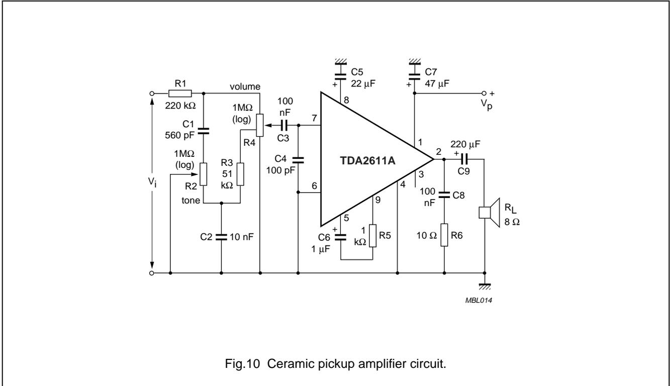
Fig.10 Ceramic pickup amplifier circuit.
